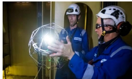
Drone surveys & remote inspection
