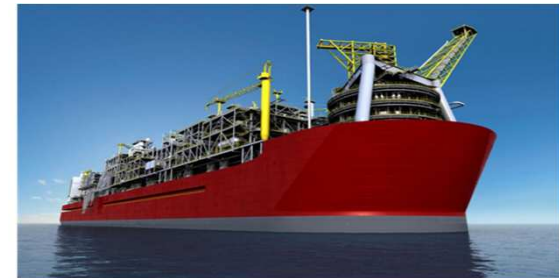
Shell Prelude FLNG, Australia, featuring two-row MkIII membrane CCS
